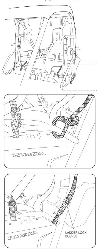
15. From the inside of the vehicle, wrap the lower inner webbing strap around the lower horizontal OPS tube, and then up through the ladder lock buckle. Repeat for the other side.
