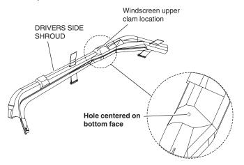
10. Attach a webbing/buckle attachment through the drilled hole in each shroud, with a large flange rivet, as shown.
