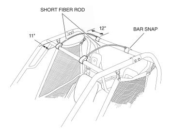
Install the fabric roof/rear panel to the P-channel by draping it over the front of the vehicle with cover rod pockets face up and slide the welting on the front edge of cover through the opening in either end of the P-channel.
