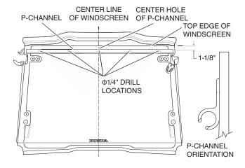
3. Install the P-channel using the 6 mm hardware provided, with each bolt and one washer inserted from the outside and with another washer and each nut installed from the inside of the windscreen. Once the P-channel has be installed, reinstall the windscreen to the vehicle. Do not fasten the upper windscreen clamps at this time.
