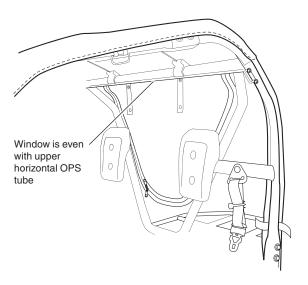
17. From the inside of the vehicle, tightly wrap the hook and loop straps around the vertical OPS tubes. Tightly wrap the hook and loop straps around the lower horizontal OPS tube.
