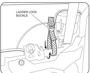
16. Tighten all of the webbing straps evenly. The top of the rear window should be even with the upper horizontal OPS tube. The bottom of the rear window should be pulled tight.
