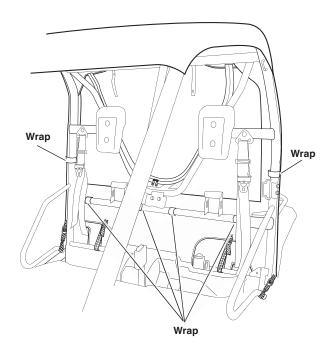
18. To ensure a tight fit after tightening rear straps, tilt the windscreen down and lock it in that closed position. The top of the wind screen will move forward and tension the cover to ensure a tight fit.
